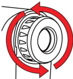
2. To focus/increase clarity, use the **Diopter Adjustment** by turning the **Eye Piece**.
