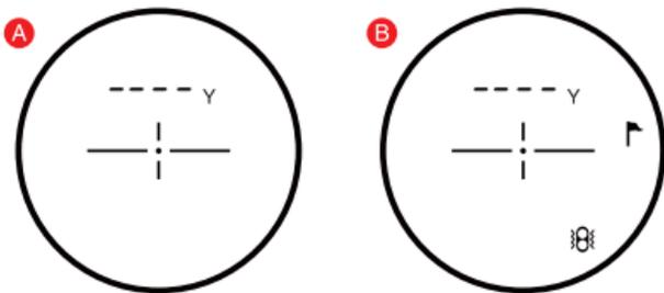
**NOTE:** To disable Pulse Technology, **TOUCH & HOLD** the **MODE** pad on the left side grip until you see a vibration icon in the bottom right corner of the LCD display. **TOUCH & RELEASE** the **PowerPad™** on top to change from **ON/OFF**.
