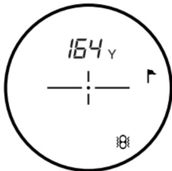
3. Continue looking through the **Eye Piece**, aim the **Center Dot** inside the **Crosshairs** at your target and **TAP & RELEASE** the **PowerPad™** on top to shoot a distance. The device will vibrate, and the distance will be displayed on the **LCD Screen**.
